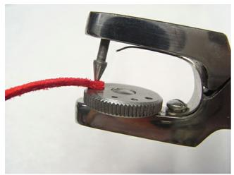
Set the hole punch to the smallest hole and line up the point 2mm (1/16") from the end of a piece of lace. Punch a hole making sure the hole is centred. Do this at both ends of every piece of suede lace.
