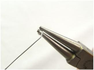
Cut three 10cm (4") lengths of wire. Coil one end of each wire.
