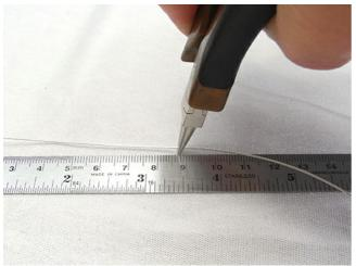
Cut a 25cm (12") length of wire. Using the round nose pliers, grip the wire 9cm (3  $\frac{1}{2}$ ") from one end.
