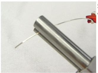
Switch to the bail making pliers. Grip the wire 20mm (3/4") from the end.
