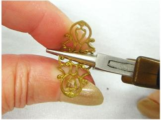
Place the centre of the filigree into the lower part of the jaws of the round nose pliers. Press your finger and thumb around the base of the filigree to round one side of it.
