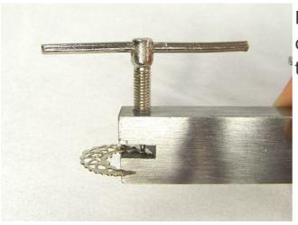
Punch a hole near the point of the crescent moon charm on one end with the metal hole punch.
