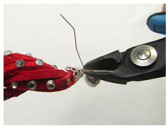
Trim away the excess wire. Slide the components up to the loop if there is a bit of a gap.
