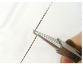
Wrap the longer end of the wire around the tip of the round nose pliers to create three complete coils.
