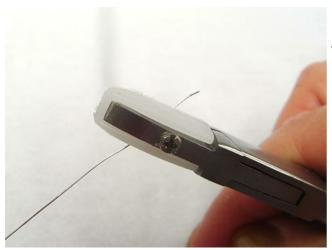
Use the nylon jaw pliers to straighten the cut end of the wire.
