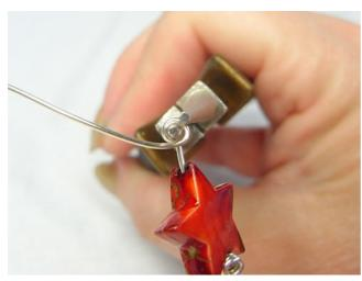
Grip the wire with chain nose pliers above the point of the star and bend it at a 90° angle above the pliers.
